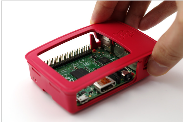
FIGURE 16-3: Assembling the top of the case
